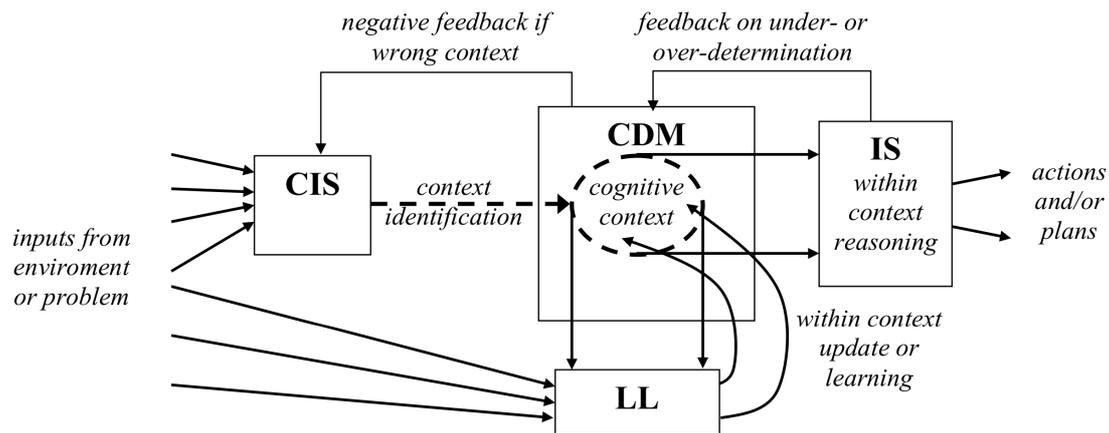
Figure 1. How the context-identification system (CIS), the context-dependent memory (CDM), the local learning algorithm (LL), and Inference system (IS) work together.
